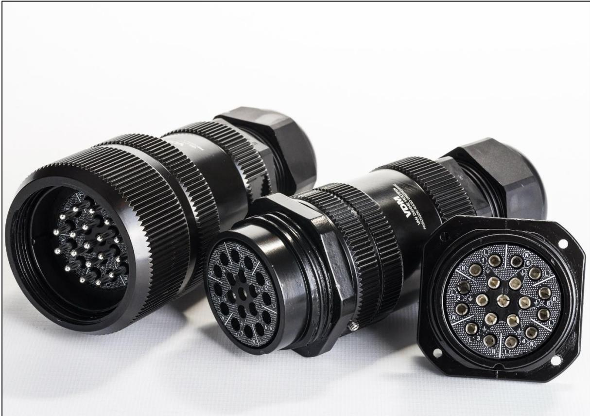
Van Damme VDM 19 pole connectors are robust, tour grade connectors for high current speaker and 6 circuit lighting power applications. They feature heavy duty machined locking rings for ease of mating, anti-rotational grub screw and insert to prevent internal wiring damage and protective forward mounted earth contacts. They are compatible with Socapex and other manufacturers' 419 series connectors.
